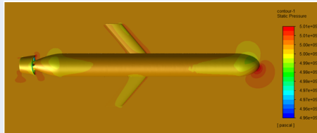
Figure 21: Pressure contour of the fluid as the AUV rotates around a fixed center in the vertical plane
