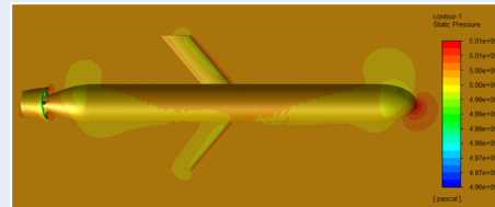
Figure 13: Pressure contour of the fluid as the AUV rotates around a fixed center in the horizontal plane
