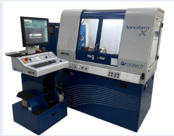
Figure 1: Ultra-Precision Turning Machine Nanoform ® X [Source: Authors]
