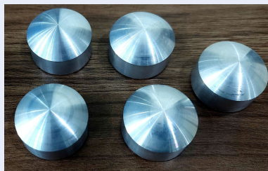
Figure 3: Al6061 Spherical Workpiece [Source: Authors]
