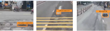
Figure 10: The software detects allocation with damage and predicts its expansion into a serious damage in the near future, Pictures made by the RTI IMS model, "Source:The authors".
