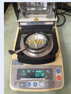
Figure 2: Moisture content analysis of samples on AND MX-50 [Source: Authors]
